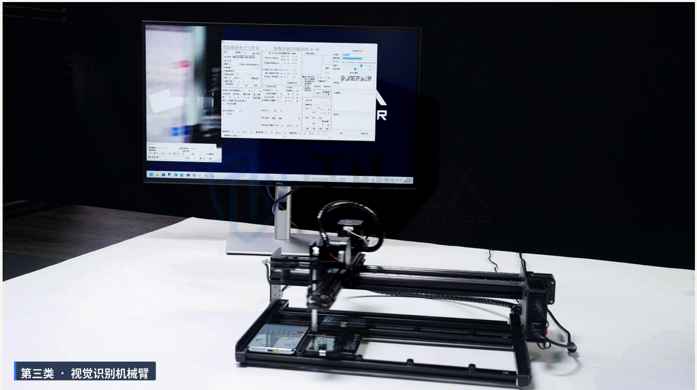
FIG. 3 Class 3 devices: a vision-guided robotic arm. A camera reads the page; a mechanical structure then makes real taps and swipes.
