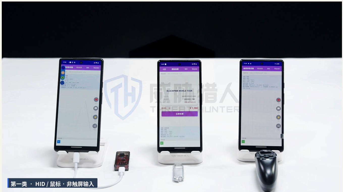
FIG. 1 Class 1 devices: HID and mouse clickers. Clicks and swipes are injected through input protocols; there is no real finger on the glass.
