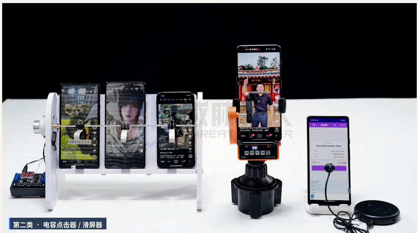
FIG. 2 Class 2 devices: capacitive clickers and mechanical sliders. Capacitive tips or mechanical structures make real contact with the screen and repeat taps and swipes.
